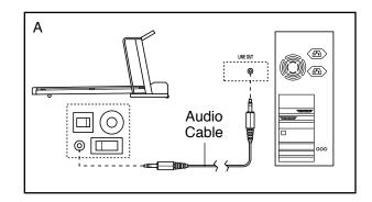
B. Plug one end of the audio cable into the jack on the front of the treadmill near the power cord. Plug the other end of the cable into a 3.5mm Y-adapter (available at electronics stores). Plug the Y-adapter into the PHONES jack on your computer. Plug your headphones or speakers into the other side of the Y-adapter.
